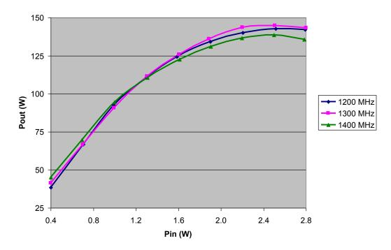
**RF Power Transfer Curve (Output Power Vs. Input Power)**
